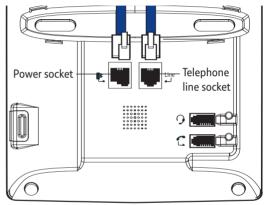
5. Press the line cables into the grooves on the base of the phone so that the phone can lie flat.
