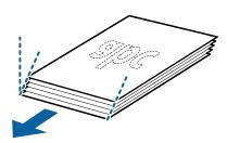
6. Load the originals into the input tray facing down with the top edge facing into the ADF.
