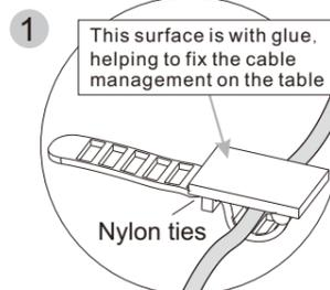
1 This surface is with glue, helping to fix the cable management on the table
