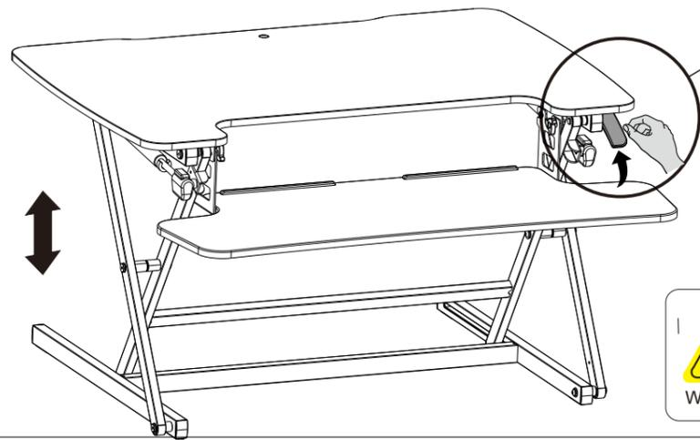
Based on the actual usage, press the handle grips simultaneously, and adjust the workstation to the proper height
