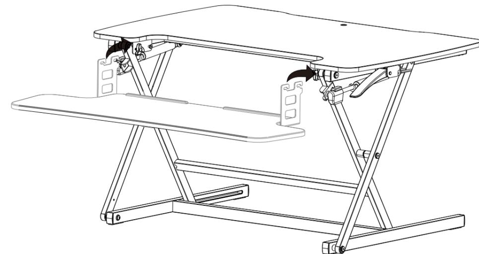
Hang the junction plate on the knob assembled and then tighten the knob
