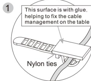
1 This surface is with glue, helping to fix the cable management on the table
